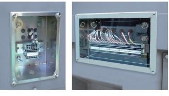
Instrument cables are routed into a single junction box and the incorporation of clamp-type terminals as standard simplifies the cable connection process. As a result, external cable connection work is simplified, reducing installation times. Furthermore, the junction box is made of stainless steel, increasing operating durability under harsh conditions.
